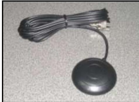
*Figura 11: Antena GPS*
