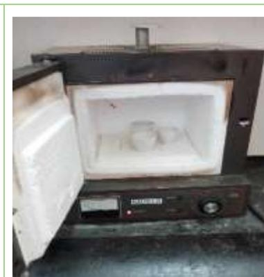
A muffle furnace with its door open, showing a crucible inside, used for ash analysis. |
