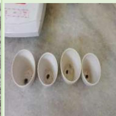
Four white crucibles containing samples, used for moisture determination.             |
