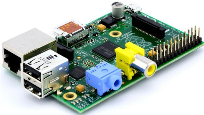
**Figura: 15: Raspberry PI Modelo B**
