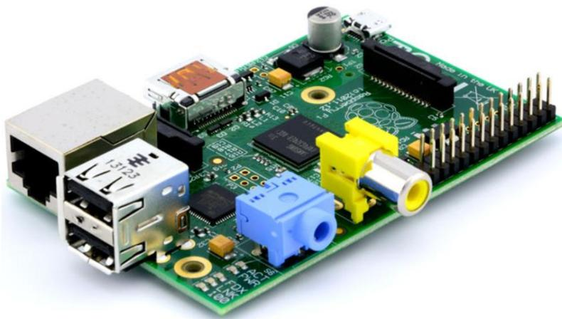
**Figura: 5 Raspberry PI Modelo B**
